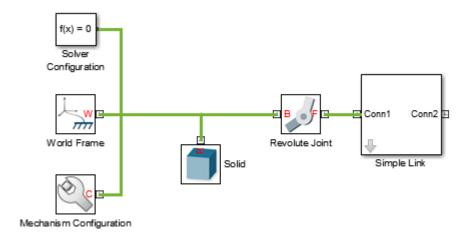
**6** In the Solid block dialog box, specify the following parameters. This block connects rigidly to the World frame and therefore has no effect on model dynamics. You can leave the inertia parameters in their default values.
